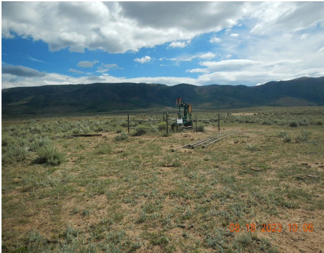
Photo #2 Fenced wellhead and pumping unit. Some tubing on the ground near well.
