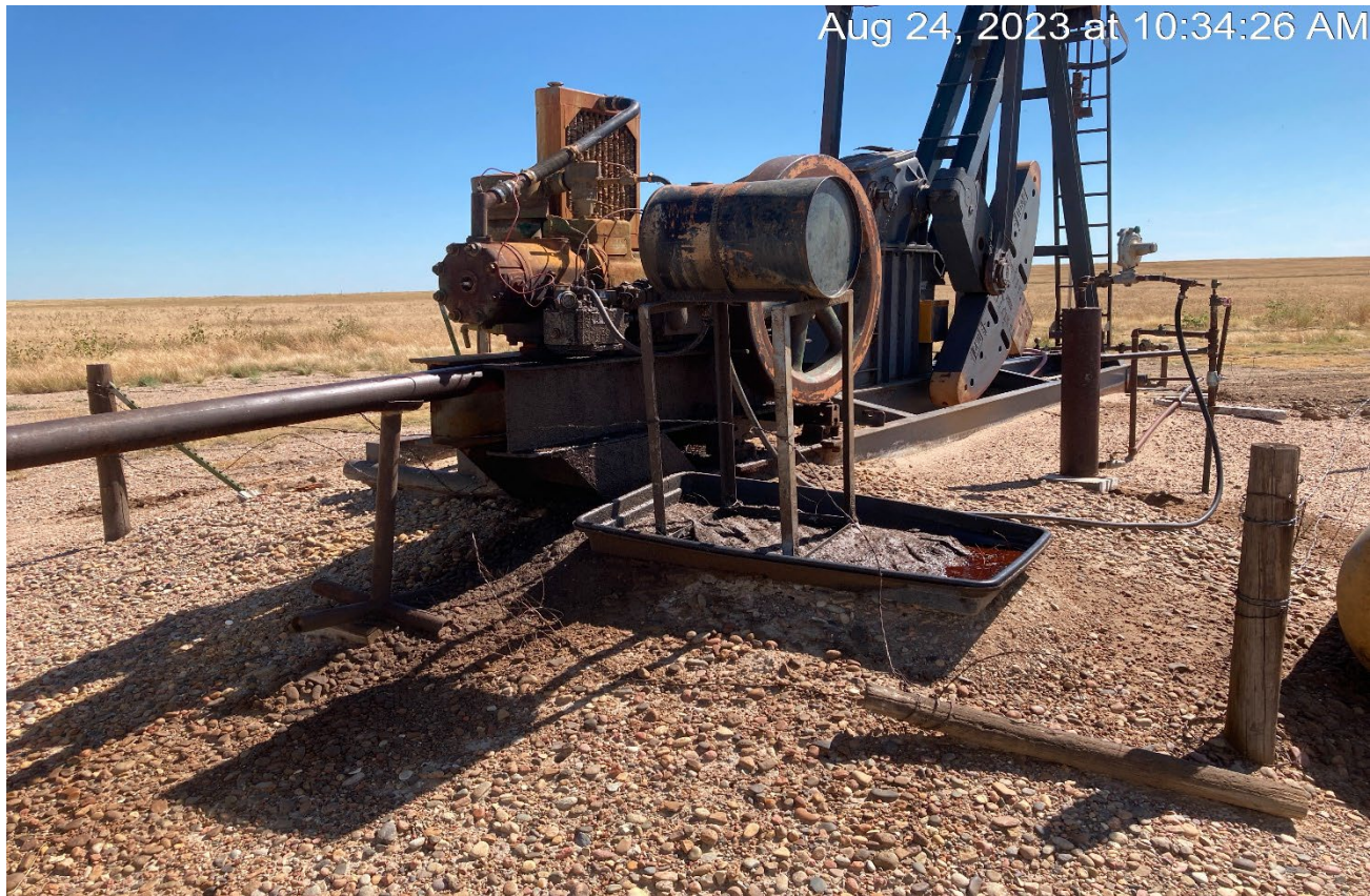
Photo 6. There is oily fluid in the containment next to the pump jack. Oily fluid has spilled onto the ground and needs to be cleaned up.
