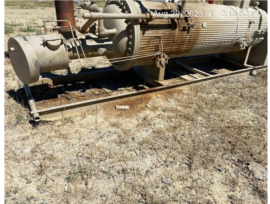
Debris. Oily waste. Stained soil
