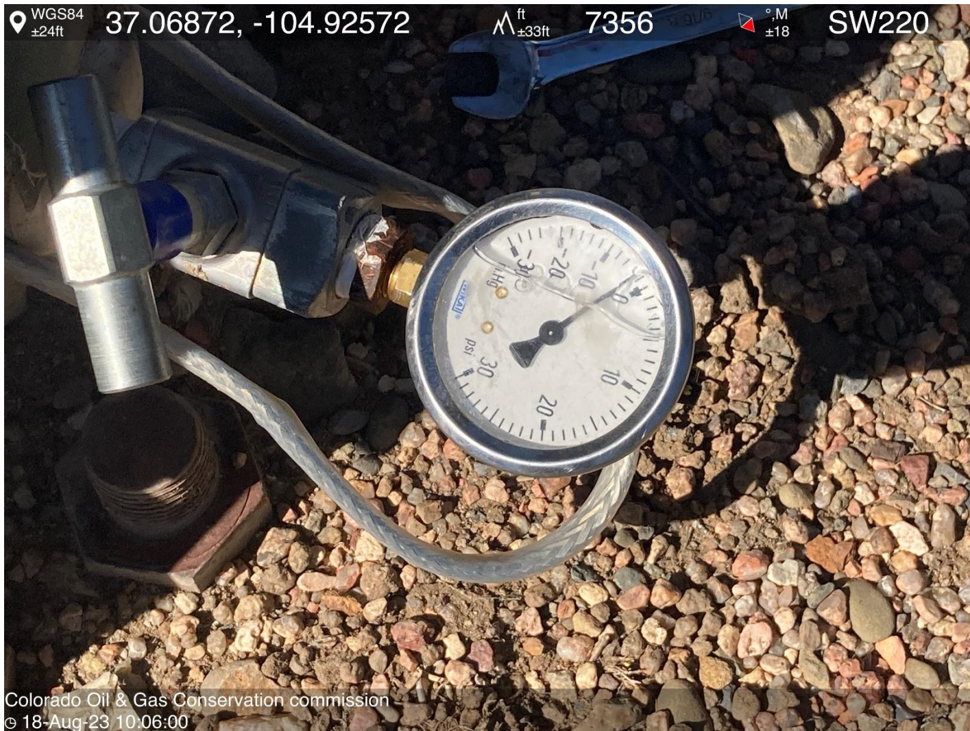
PHOTO 5: T-C PRESSURE -2 PRESSURE EQUILIZED IN 3 SEC. PRESSURE DID NOT BUILD WHILE MONITORING FOR 15 MIN.
