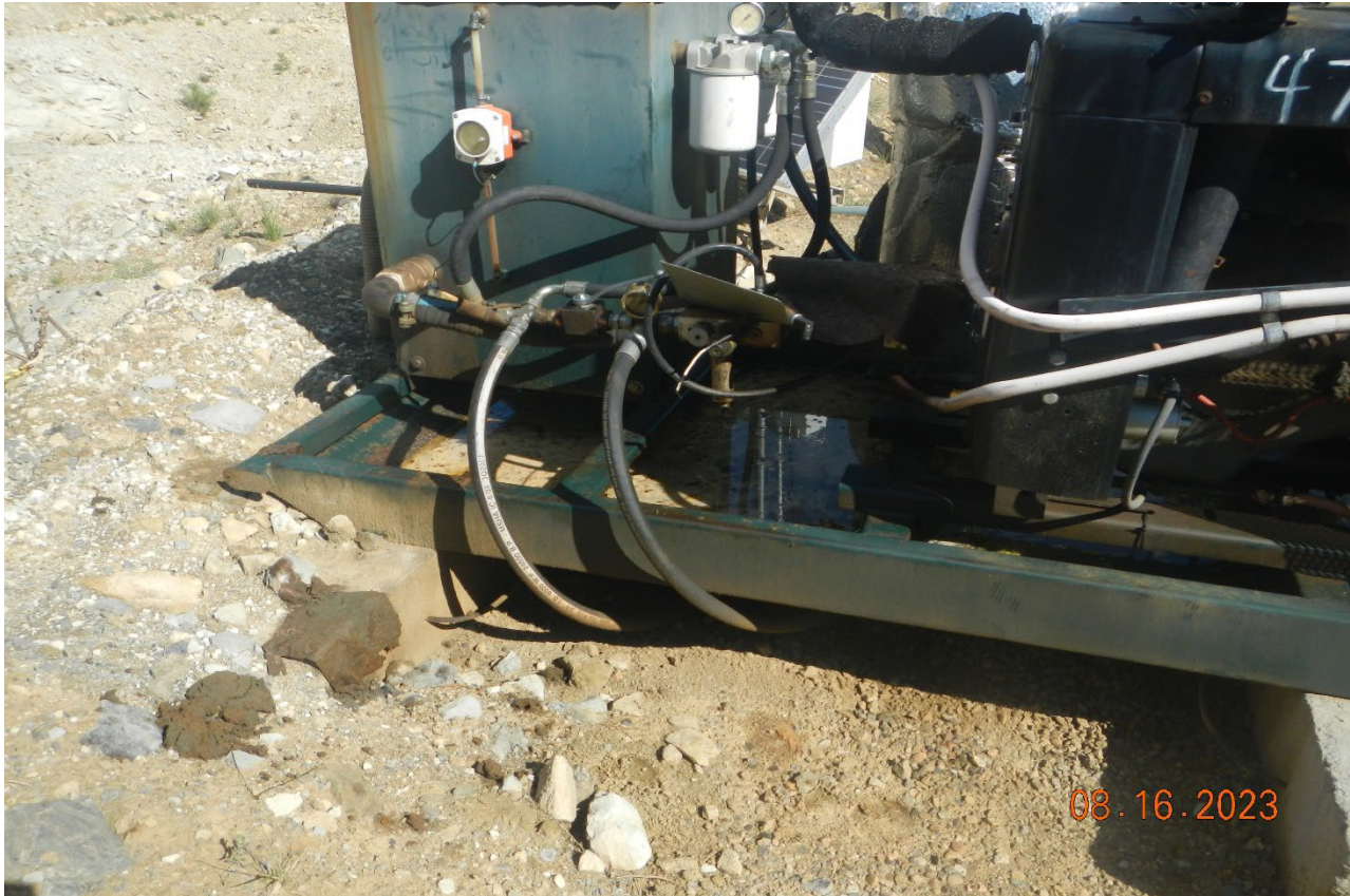
Photo 4. There are oily fluids in the engines skid that needs to be cleaned up.
