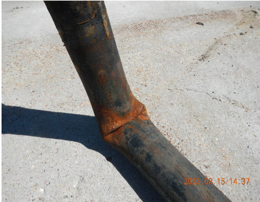
3. View of removed bent tubing joint where the tubing had split allowing the well to vent uncontrolled.
