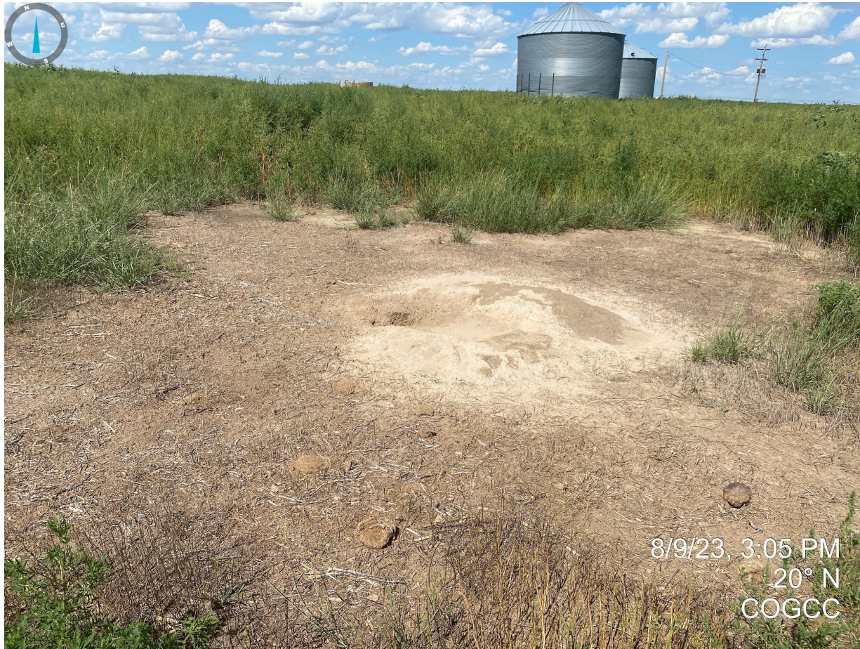
Photo 4. The former well location does not appear to be progressing towards Rule 1004 reclamation standards. Evidence of bare/exposed soil was observed, possibly a result of compaction issues or soil suitability exceedances. Further soil investigation and/or reclamation activities are required.
