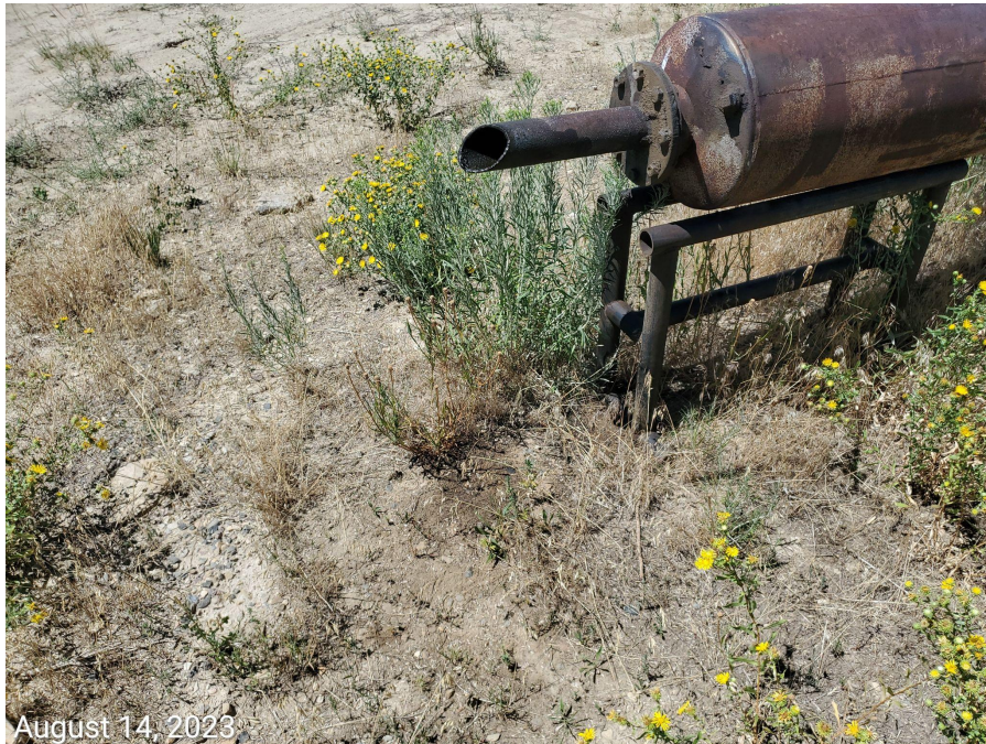
Photo 5: Stained soils observed below muffler, and at the base of the pump-jack.
