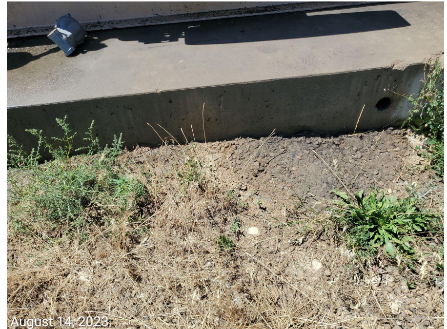
Photo 5: Stained soils observed below muffler, and at the base of the pump-jack.
