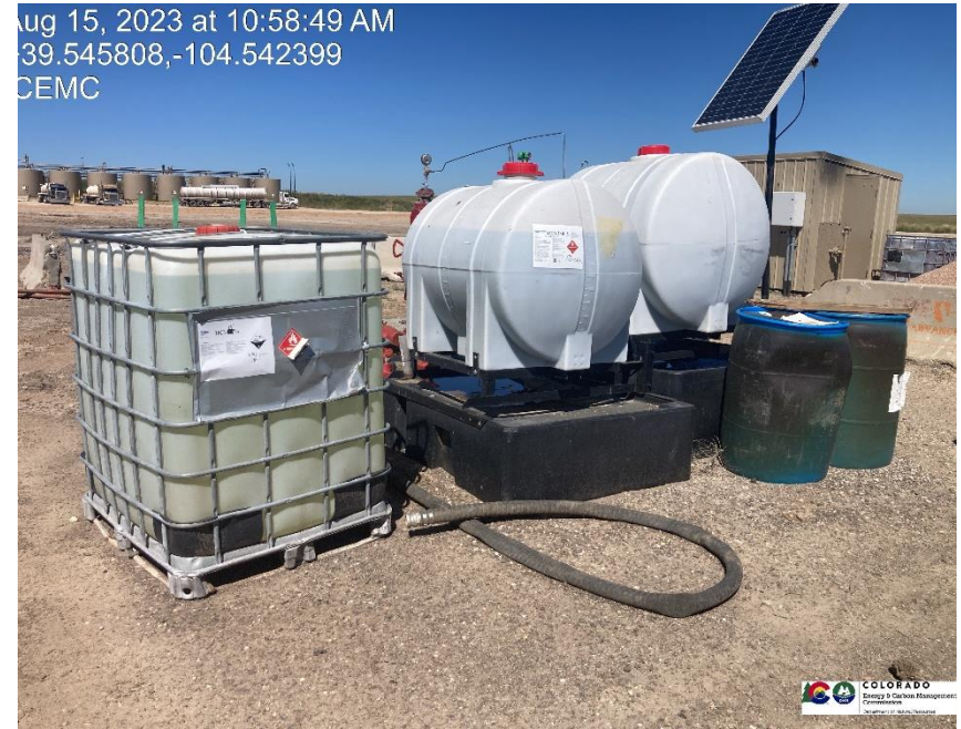
Pic 4 no control measures under chemical tanks.
