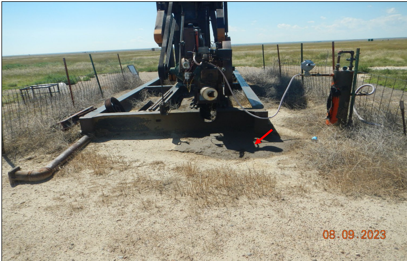
Photo 5. There is oil stained soils shown at red arrow that need to be cleaned up..
