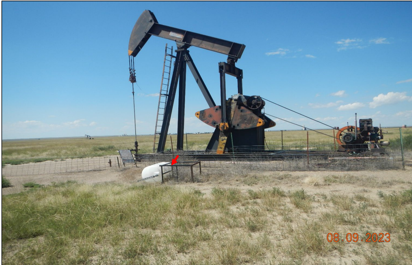
Photo 4. Facing toward the pumpjack. The chemical container has fallen over and does not have secondary containment.
