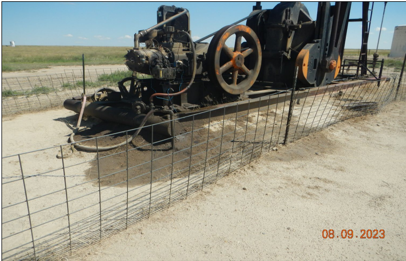
Photo 2. There are oil stained soils at the base of the pumpjack that need to be cleaned up.
