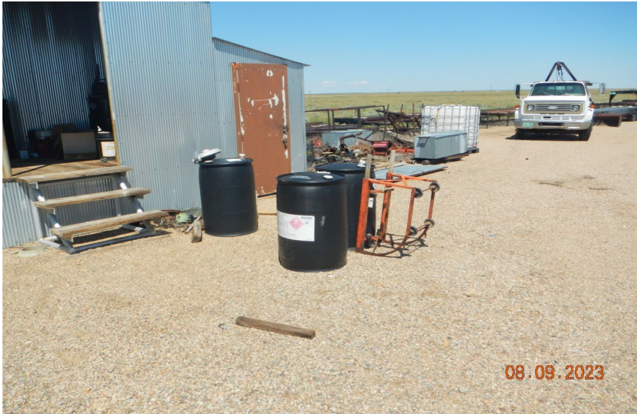
Photo 15. There are several chemical barrels on location with faded labeling and no secondary containment. Various pipe, supplies and debris stored on location.
