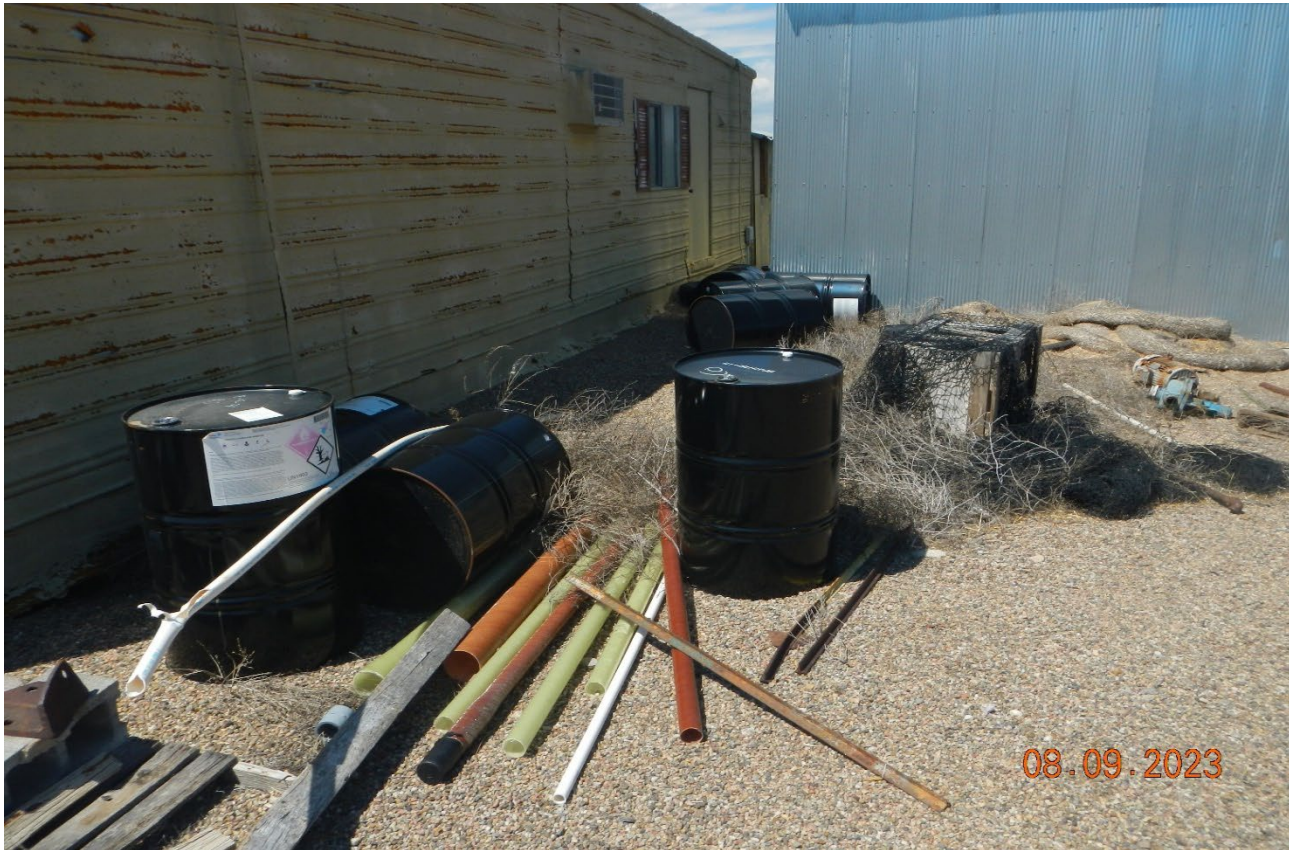
Photo 14. There are several chemical barrels on location with faded labeling and no secondary containment. Various pipe, supplies, and debris stored on location.
