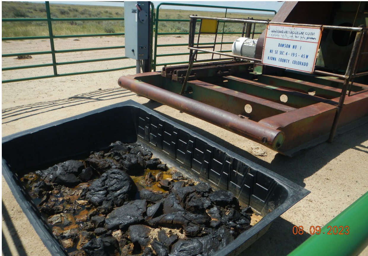
Photo 4. There is oily material being stored in this containment which needs to be removed and properly disposed. This is a potential stormwater and wildlife impact that needs to be removed.
