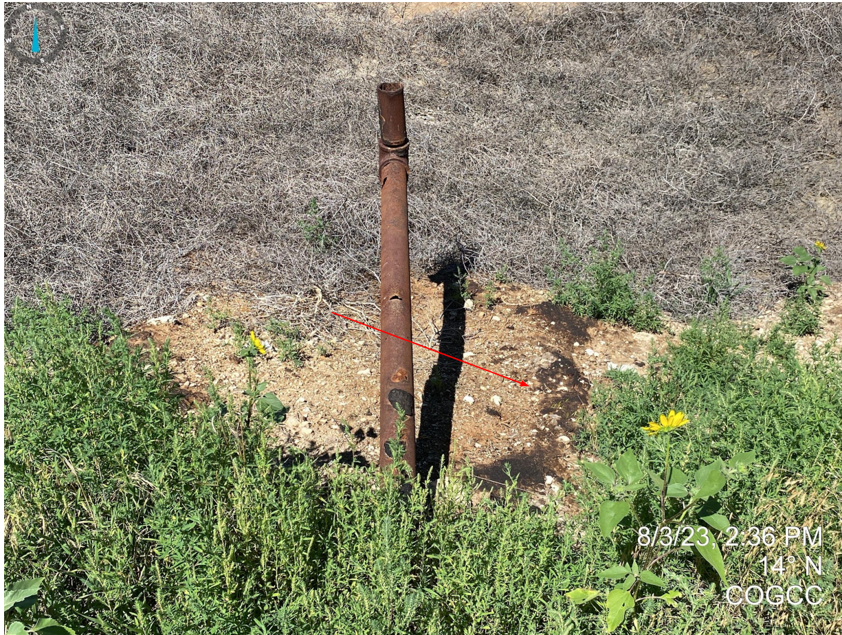
Photo 6. Stained soil observed within the skim pit. Refer to FIRs (Doc #701603755 and #709100070) for additional information.
