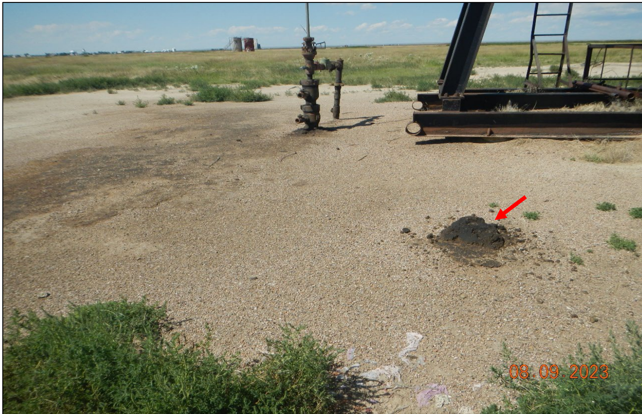
Photo 7. Facing toward the wellhead. There is oil stained soils around the wellhead which needs to be cleaned up. Area impacted is approx. 20ft.x8ft. There is oil sludge shown at red arrow.
