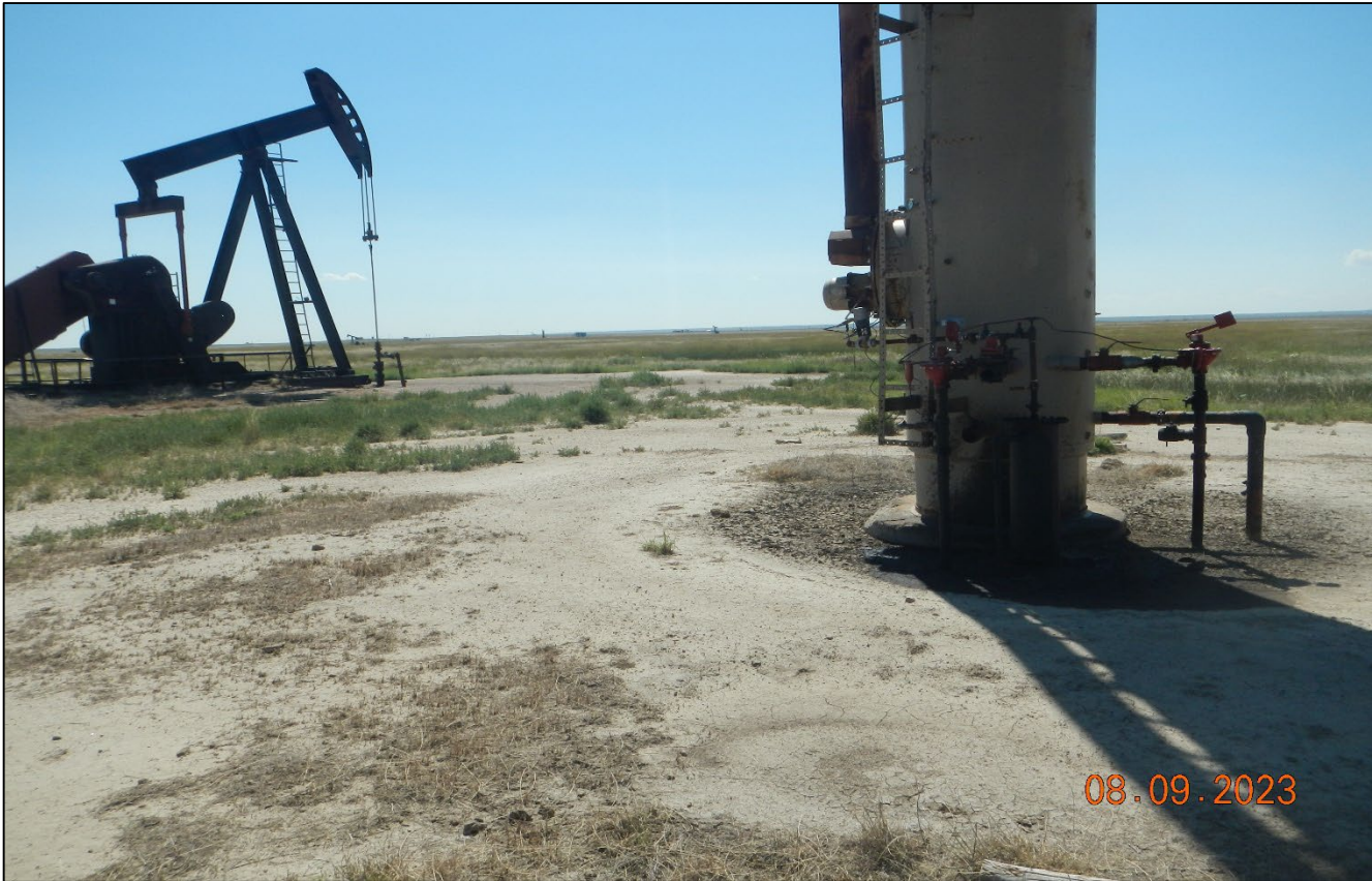
Photo 3. Facing southwest toward the pumpjack and vertical separator. There is no secondary containment around the separator tank.
