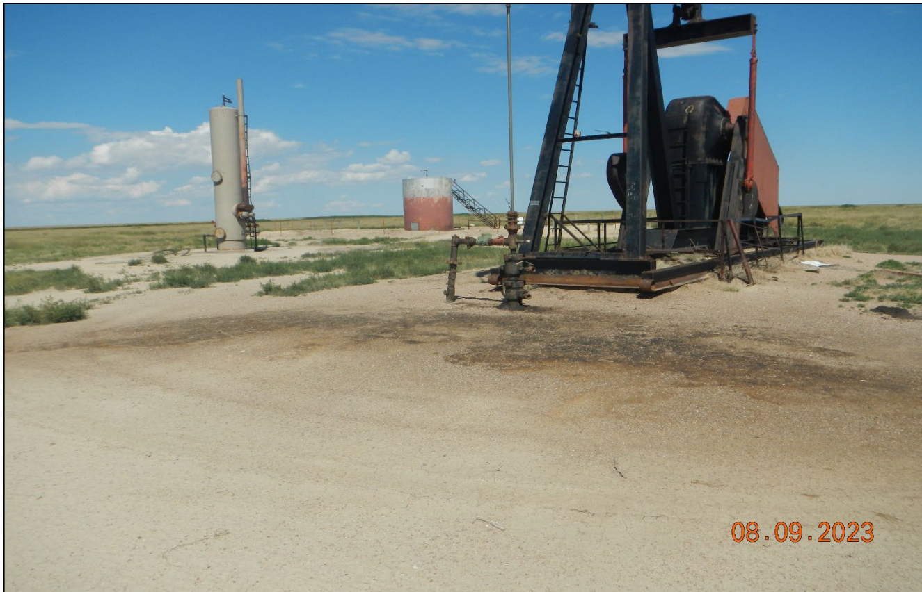
Photo 6. Facing toward the wellhead. There is oil stained soils around the wellhead which needs to be cleaned up. Area impacted is approx. 20ft.x8ft.
