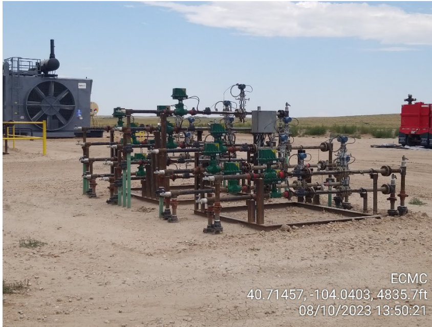
Photo 13 – Gas Lift Injection Meters
