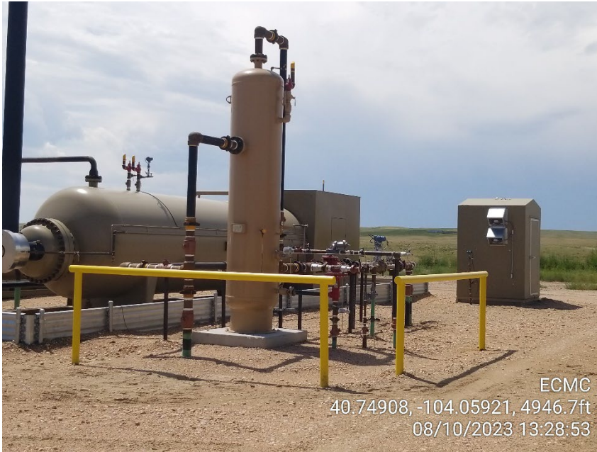
Photo 9 – Separator and Air Unit
