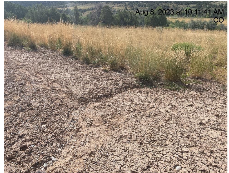
Photo # 5199 Erosion & transport of sediment off location into vegetation (near production separators)
