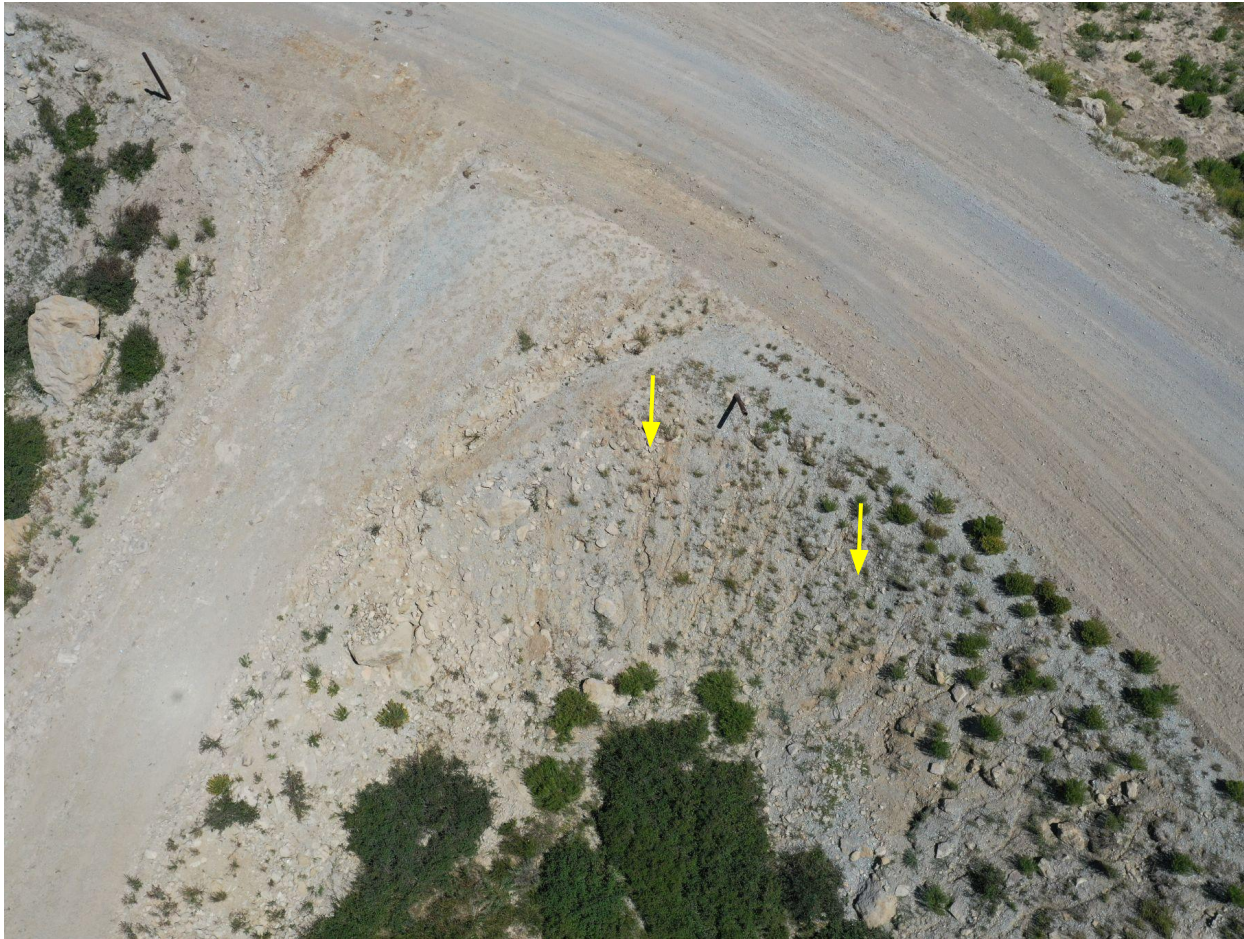
Photo 4: Photo taken with a sUAS. Photo shows erosion degradation along cut slopes. Stormwater and Erosion control measures remain missing or insufficient to manage runoff in a manner that minimizes erosion, degradation and sediment transport. Slopes/Reclamation not progressing towards 1003 standards.
