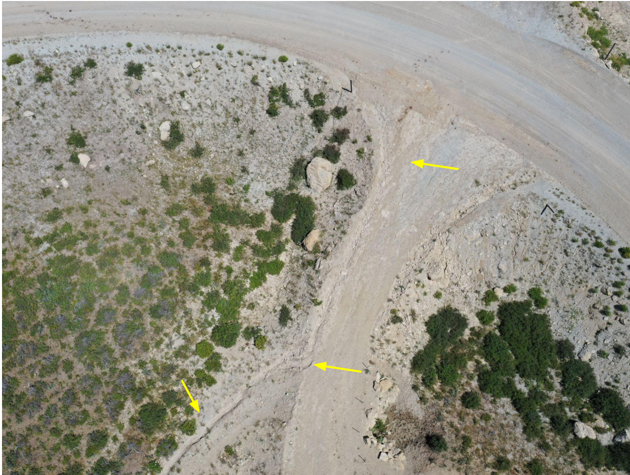
Photo 3: Photo taken with a sUAS. Photo shows erosion degradation along access road. Stormwater and Erosion control measures remain missing or insufficient to manage runoff in a manner that minimizes erosion, degradation and sediment transport.
