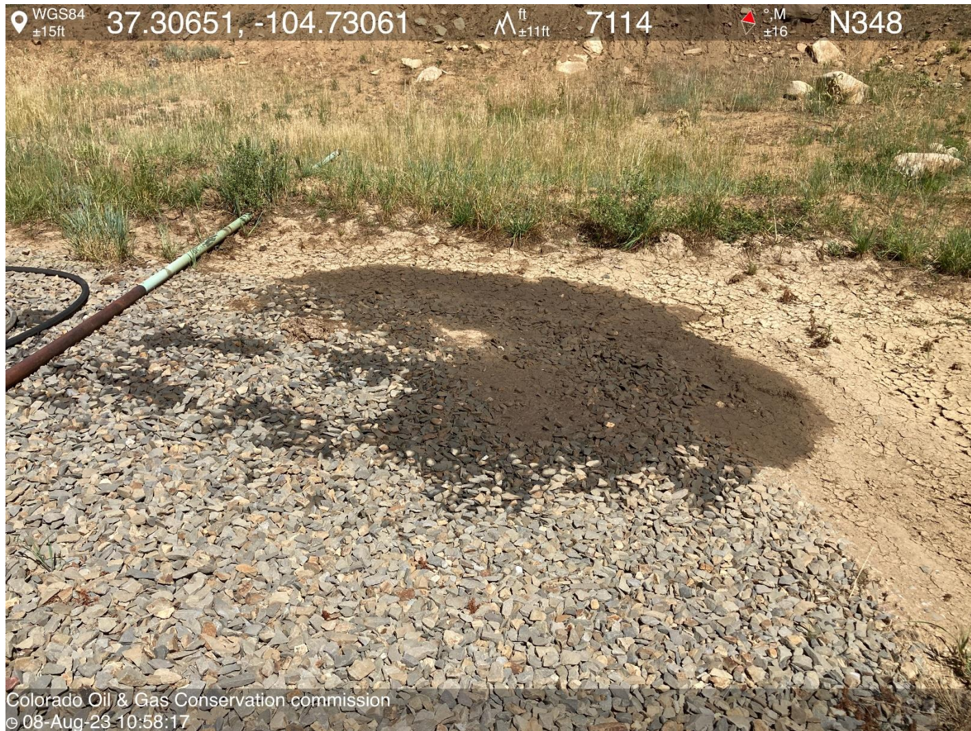
PHOTO 4: AREA OF IMPACTED SOIL BETWEEN WELLHEAD AND PIT. Conduct maintenance on equipment, cleanup stained material and review self inspection processes. COMPLY WITH RULE 1002,.(2).D. CA DATE 9-9-2023.
