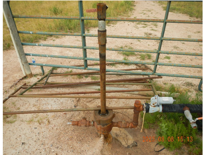
2. View of Wellhead. Note Pump Jack barrier rails on Wellhead.
