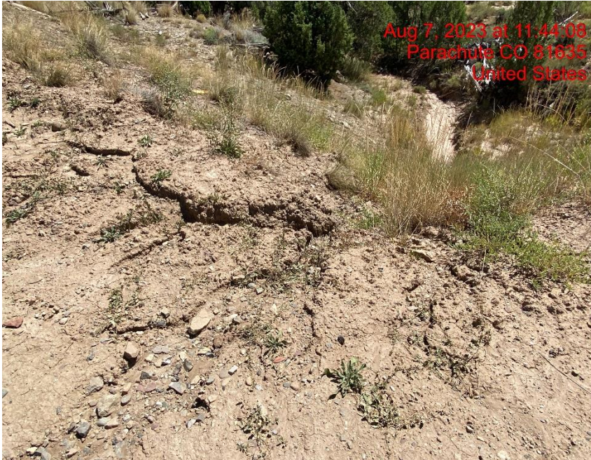
Rill Erosion Transporting Sediment to Nearby Watershed – Photo #05556
