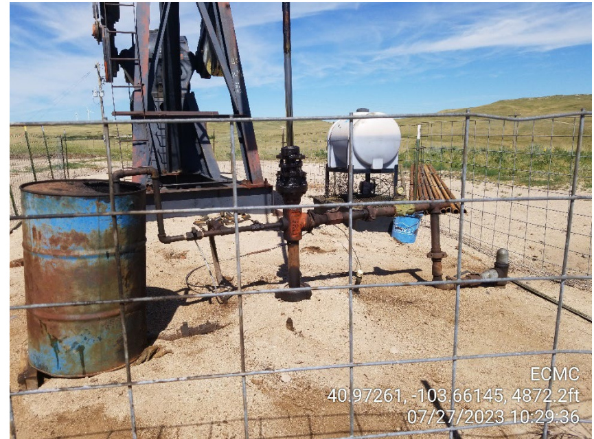
Photo 2 – Wellhead – Stained Soil
