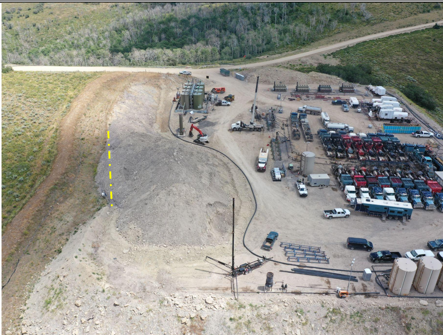
Photo 7: Drone imagery of the Location. Photo shows Operator has pushed cutting material beyond the working pad surface and cutslope (dotted line).
