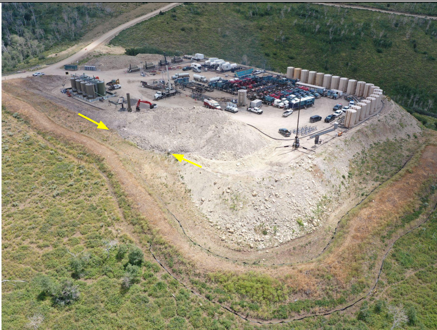
Photo 6: Drone imagery of the Location. Photo shows Operator has pushed cutting material beyond the working pad surface and cutslope (arrow).
