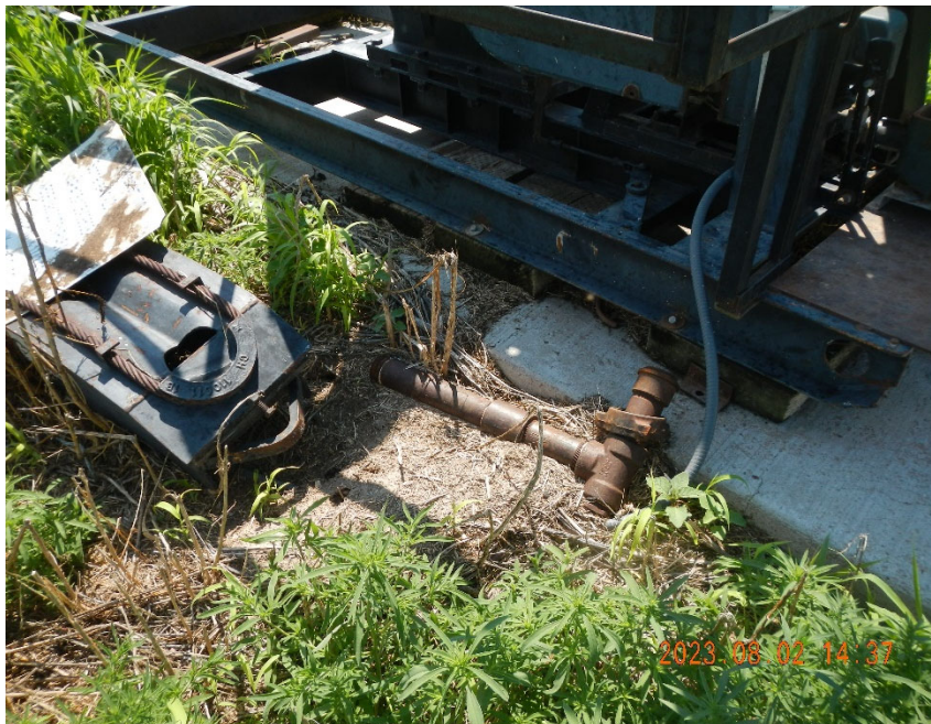
3. View of Horsehead off Pump Jack. Note vegetation.
