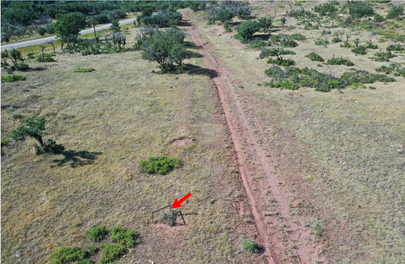
Photo 1. Drone aerial photo facing southwest toward the access road which is not reclaimed. There is a pipeline riser that has not been removed shown at red arrow.
