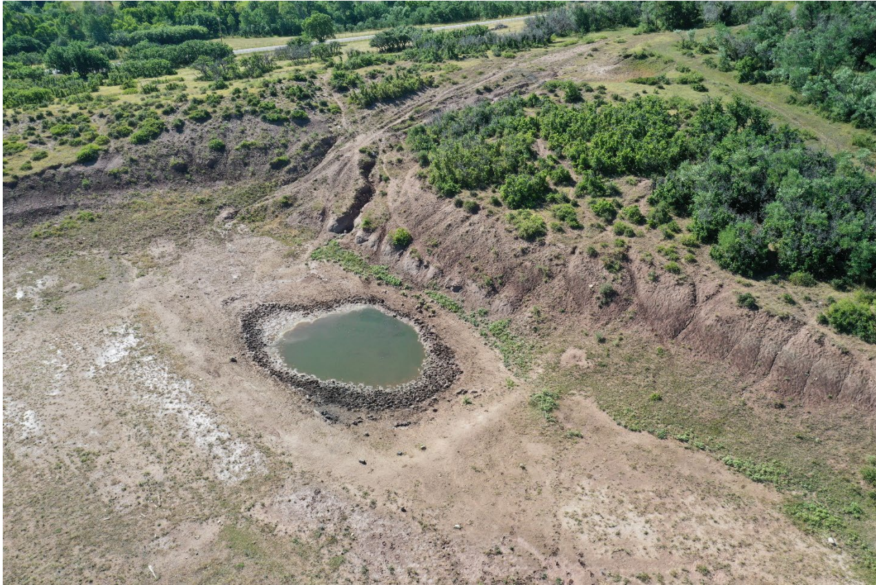
Photo 7. Facing southeast toward the cut slope which has signs of erosion gully's and rills.
