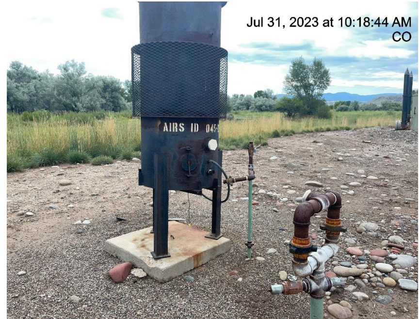
Photo # 4223 Unused equipment/ECD is disconnected
