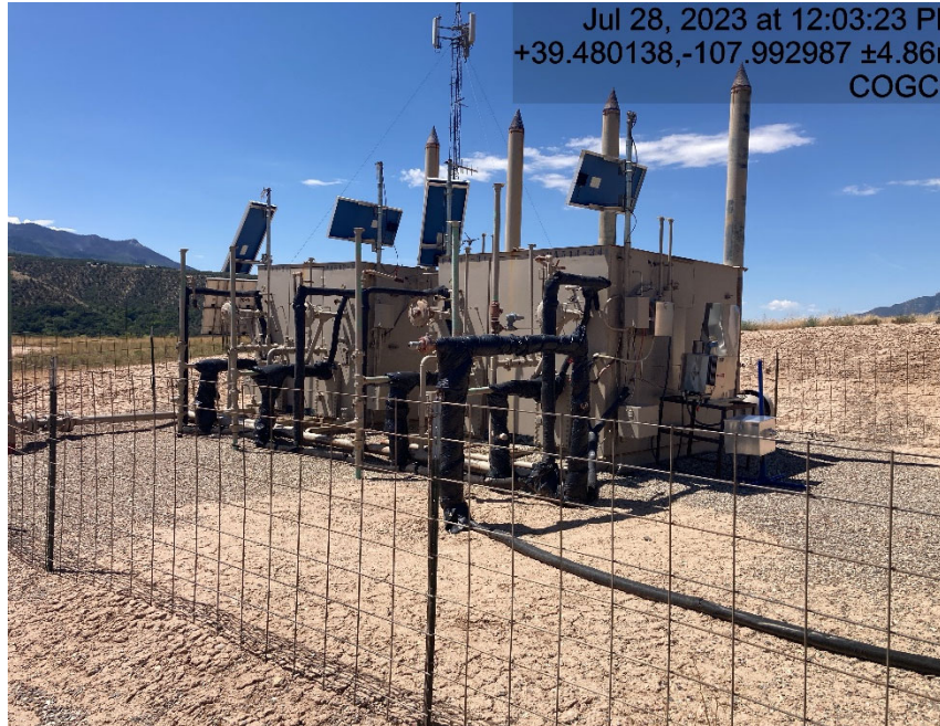
Separators and lack of access to calibration cards
