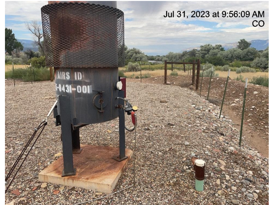
Photo # 4191 Unused equipment/ECD is disconnected
