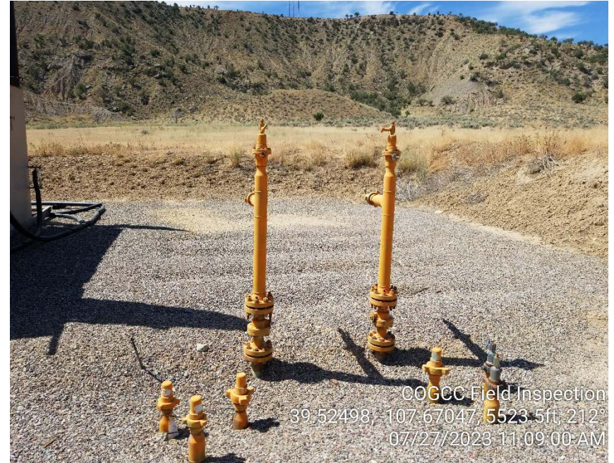
Photo #8 – Multiple marked, unused flowline risers located west of separator battery.
