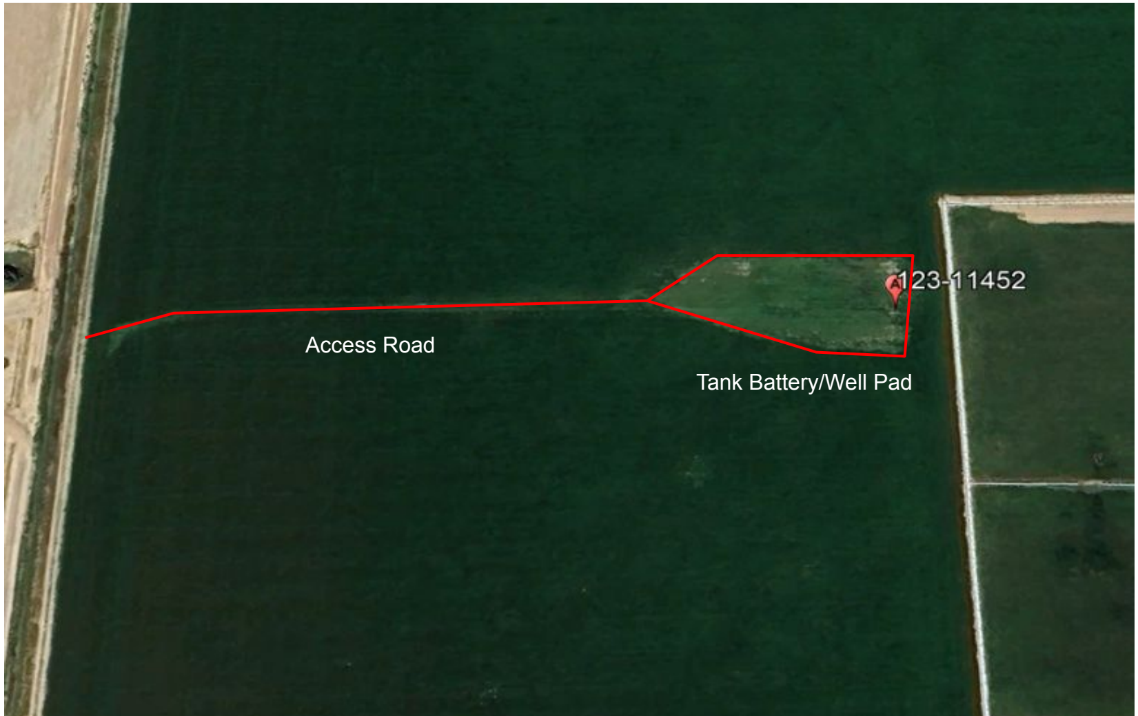
Photo 1. 2023 aerial imagery of the access road, tank battery and well pad (north is up). Note: well pad and tank battery share a disturbance area.
