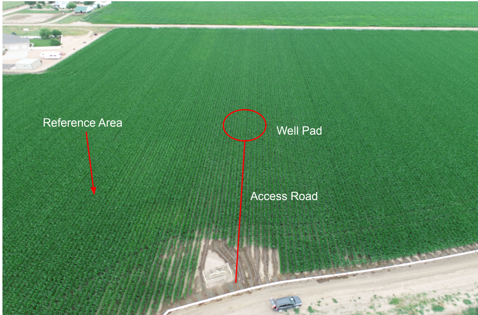
Photo 2. Overview photo of the well pad and access road. Note: well pad appears consistent with adjacent crop reference area. Riser to the south of the well disturbance was built 3 years after the well was plugged and abandoned and is not associated with PDC oil and gas operations.
