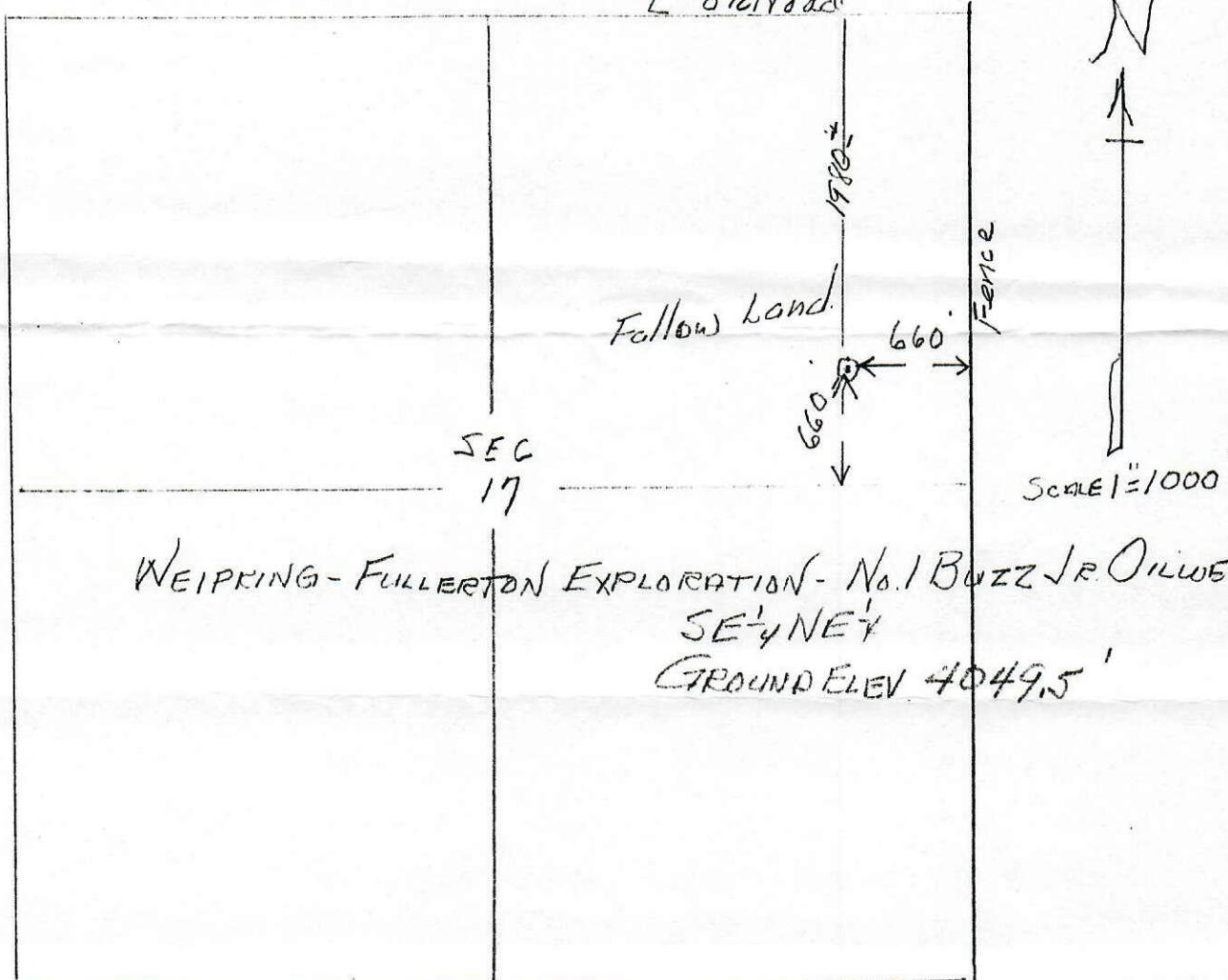
I hereby certify that the above plat is an accurate representation of a correct survey showing the location of Weipking, Fullerton Exploration No. 1 Buzz Jr. Oilwell in SE<sup>1</sup>/4 NE<sup>1</sup>/4 Sec. 17 T19S R47W 6PM. The elevation of the ground at the stake is 4049.5 feet above sea level from U.S.G.S. Bench Mark.
