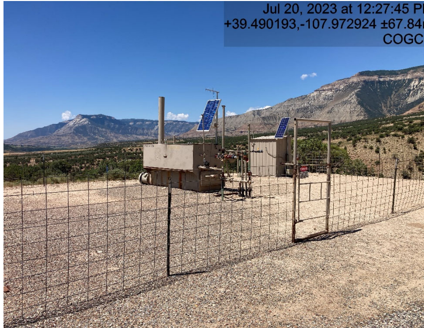
Separators and lack of calibration card access
