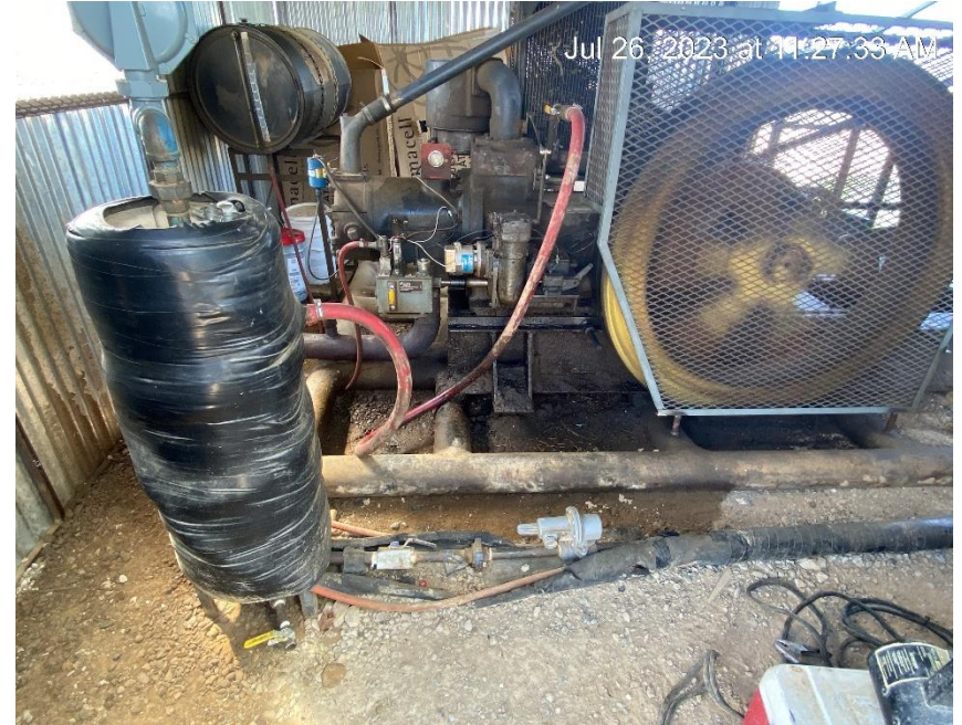
Leaking equipment and stained soil
