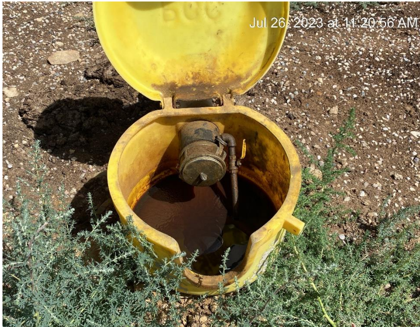
Open end loadline. Capped but valve left open
