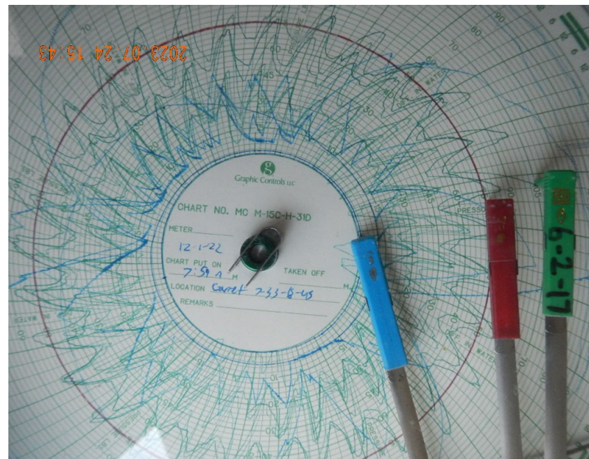
6. Chart in Meter Box at time of inspection dated 12-1-22.
