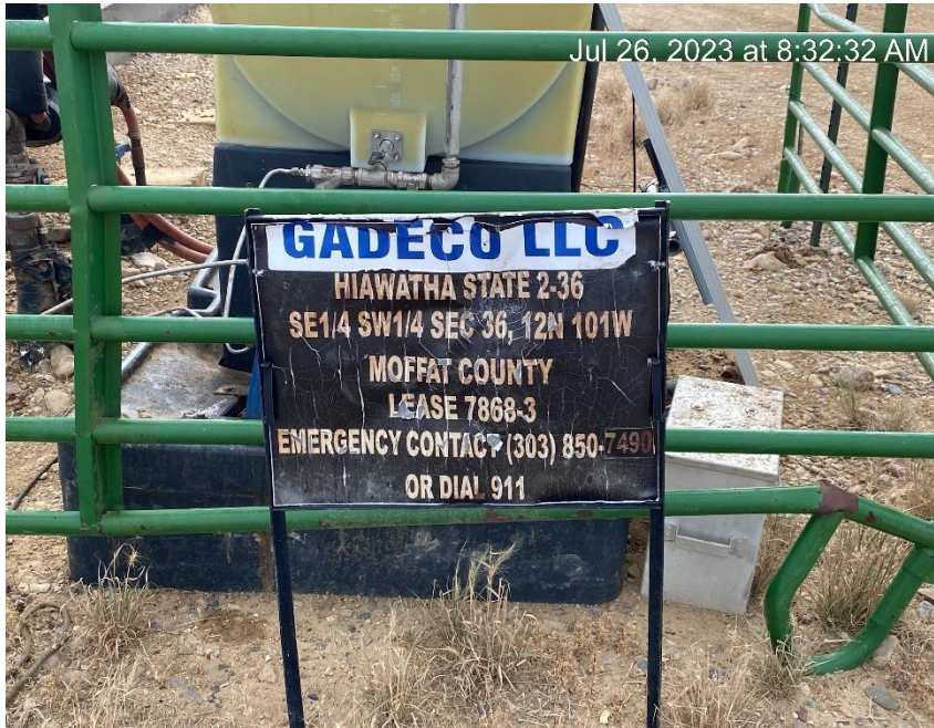
Sign at wellhead missing required information
