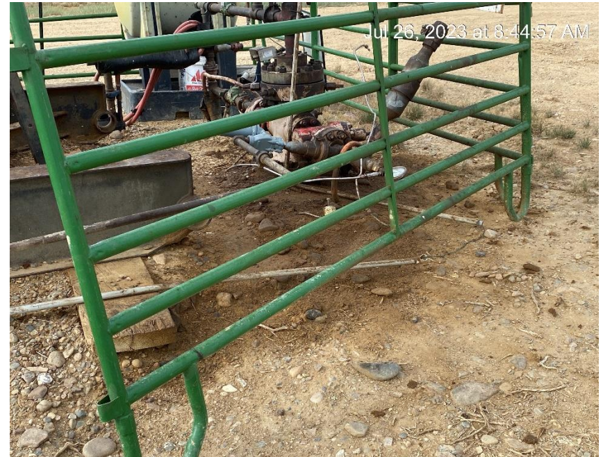
Stained soil around wellhead
