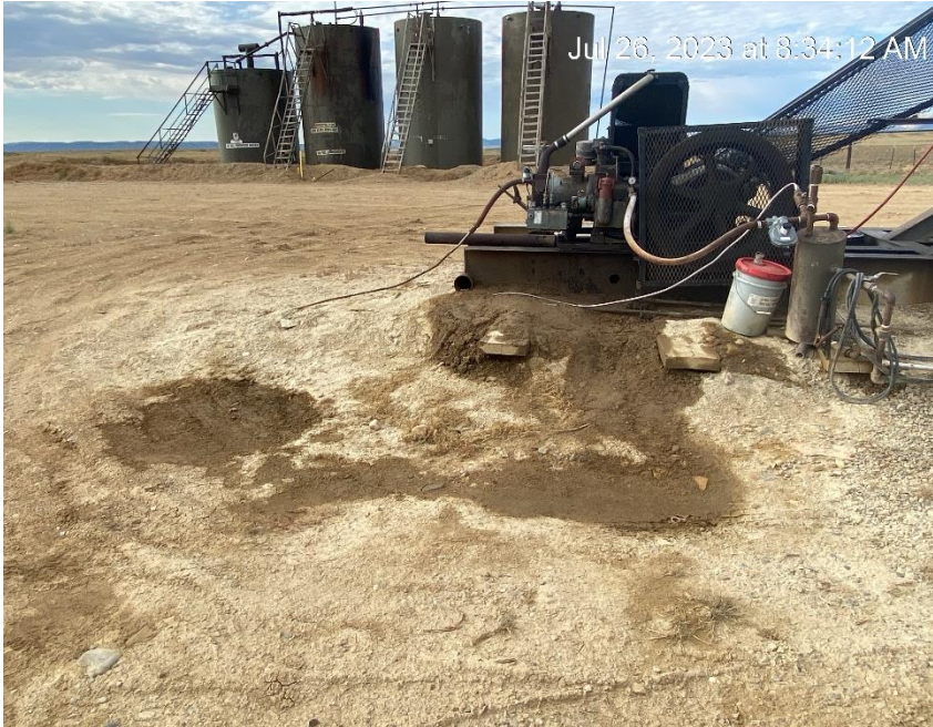
Leaking equipment and stained soil
