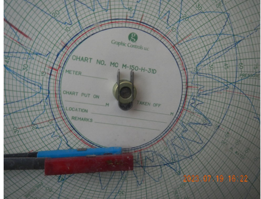
6. Undated Chart installed in Meter Box at time of inspection.
