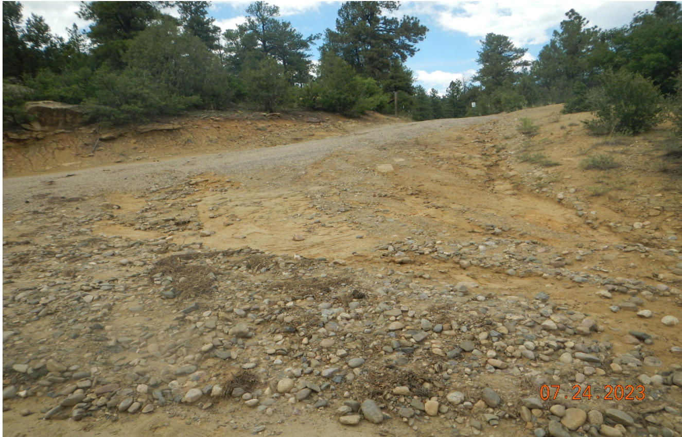
Photo 1. Facing north at the access road. There is erosion from the access road which is transporting sediment towards the County Road.
