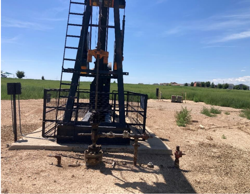
Pic 1 wellhead
