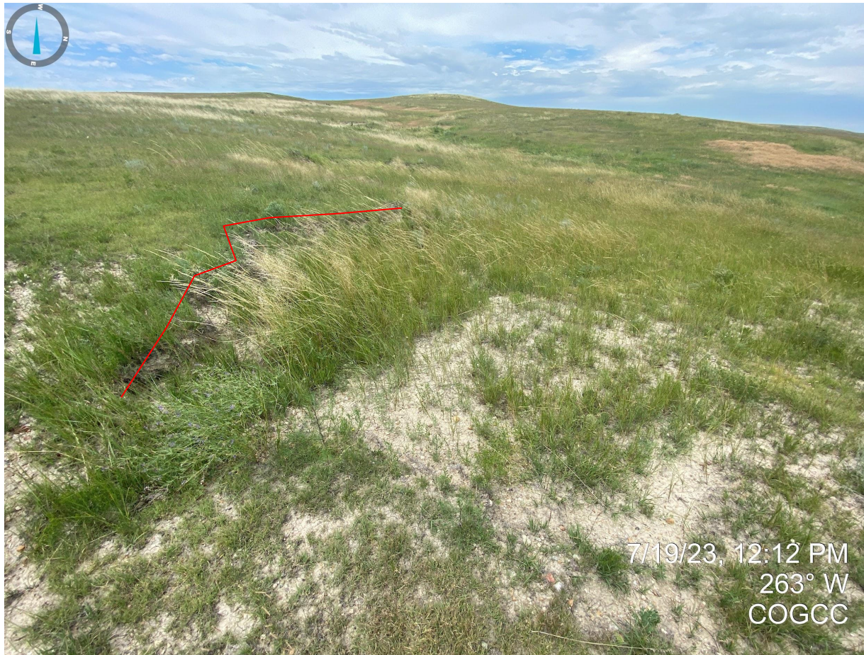
Photo 1. Taken from the former access road, facing west. Photo illustrates that cut banks (red line) have not been recontoured and bare/exposed soils are evident. Additional reclamation work will need to be performed in order to stabilize the exposed soils.
