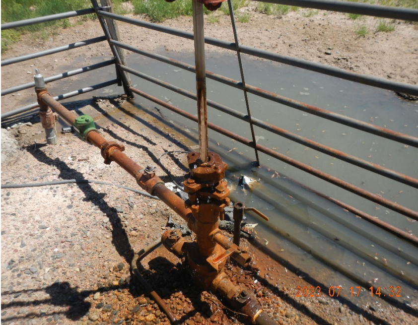
3. View of wellhead and released produced water outside fencing.
