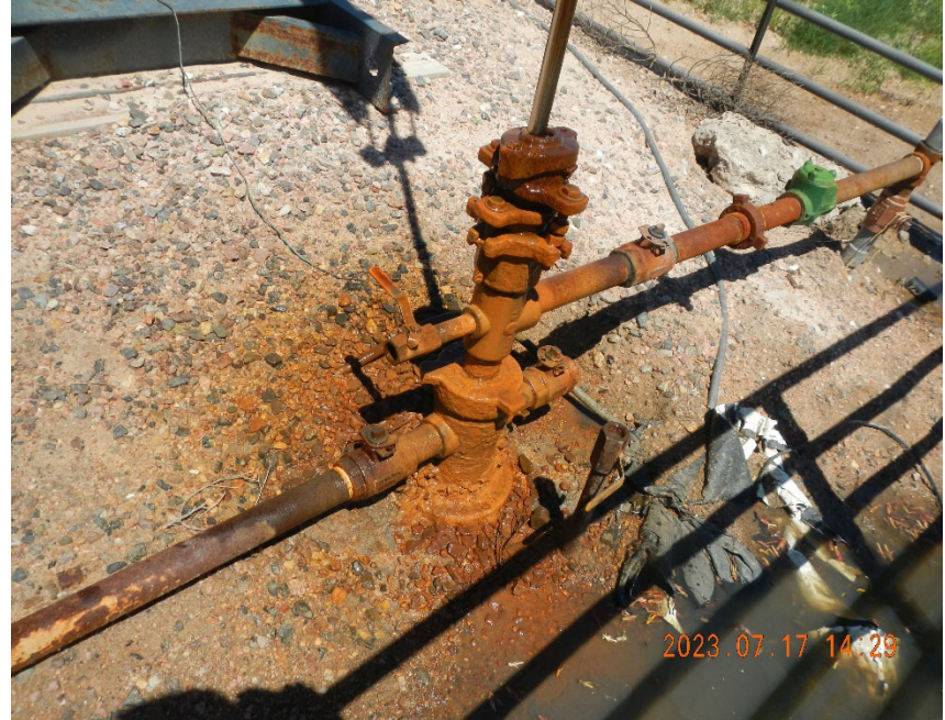
2. Wellhead. Note staining around well.
