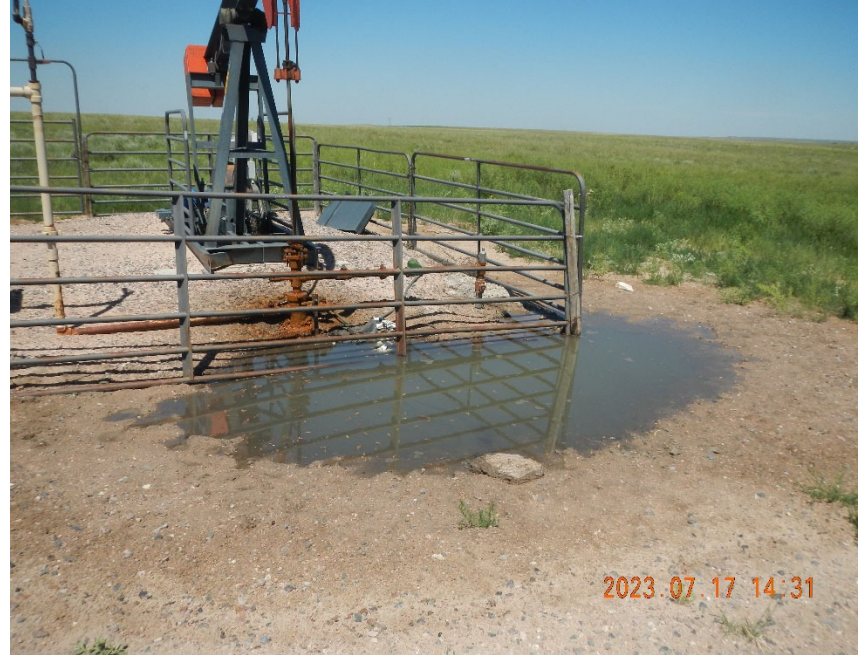
4. View of produced water released from well. Standing fluids and damp ring extending out from source.
