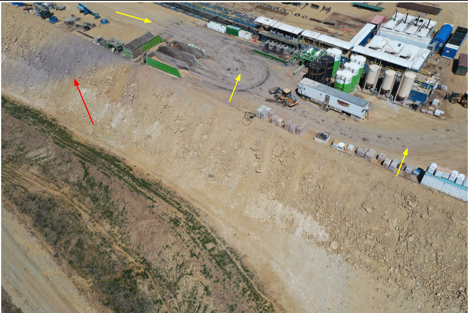
Aerial image showing spill on the fill slope (red arrow), and the drill cuttings spilled onto the working pad surface, and tracked (yellow arrows)
