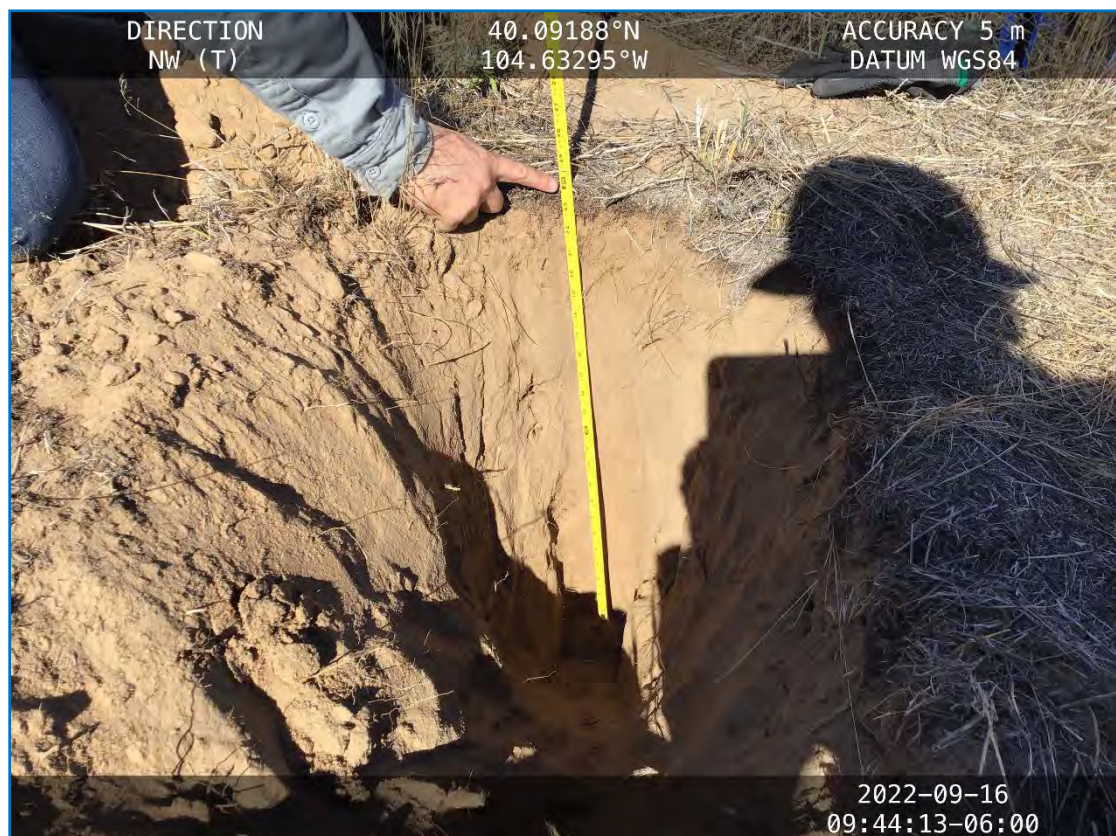
Photograph 2. Topsoil depth pit (S02); depth greater than 2 feet. Soil sandy throughout pit, with no change in color or texture.
