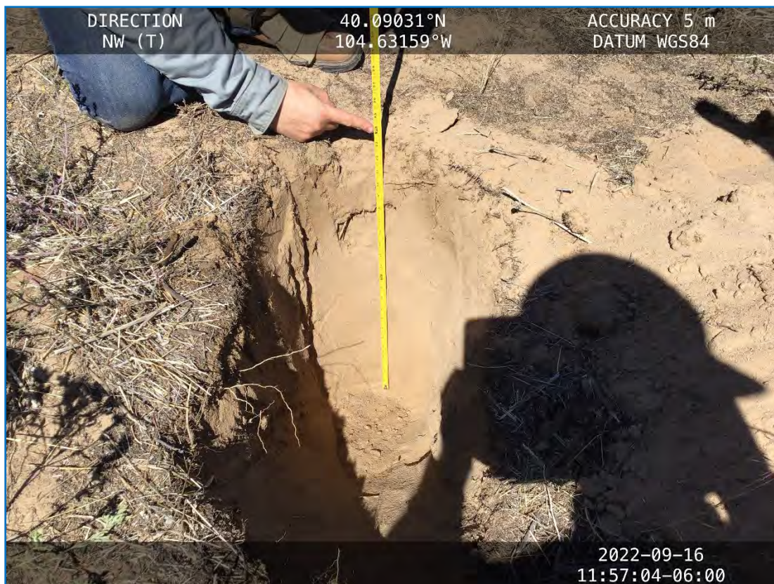
Photograph 8. Topsoil depth pit (S08); depth greater than 2 feet. Soil sandy throughout pit, with no change in color or texture.
