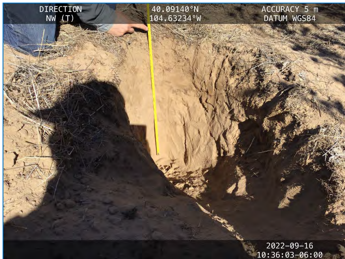
Photograph 4. Topsoil depth pit (S04); depth greater than 2 feet. Soil sandy throughout pit with, no change in color or texture.
