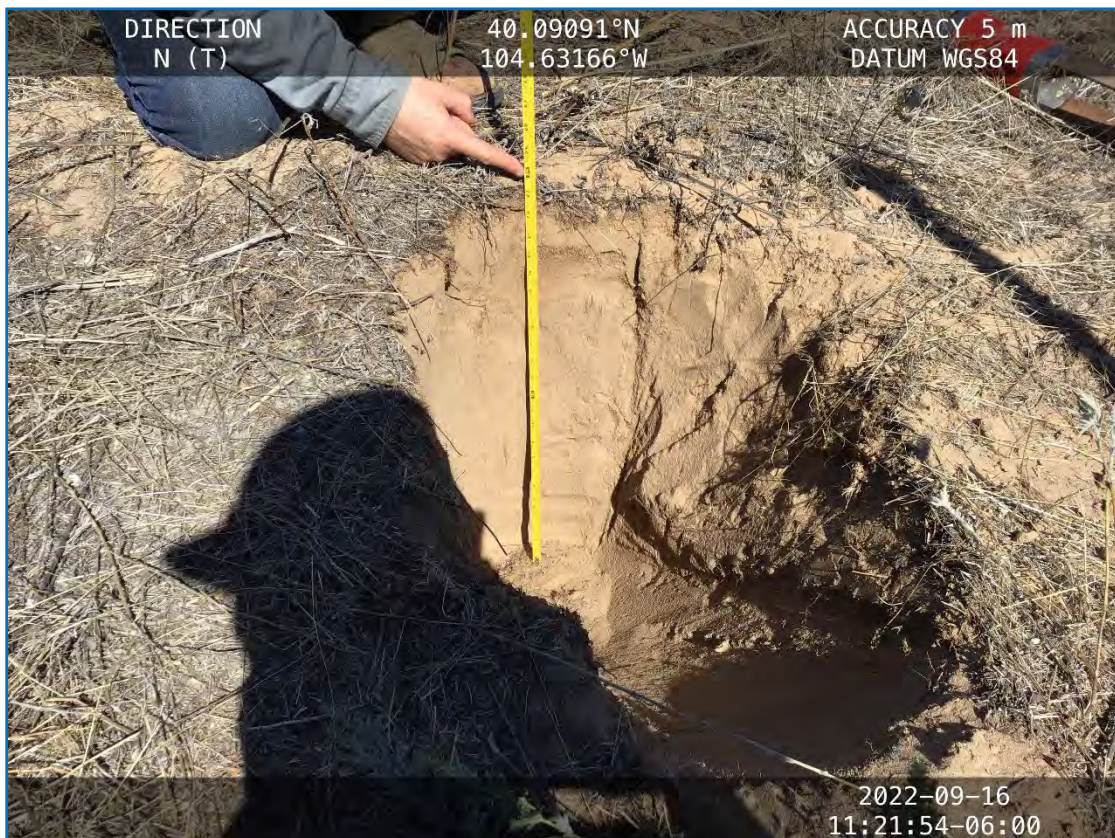
Photograph 6. Topsoil depth pit (S06); depth greater than 2 feet. Soil sandy throughout pit with, no change in color or texture.
