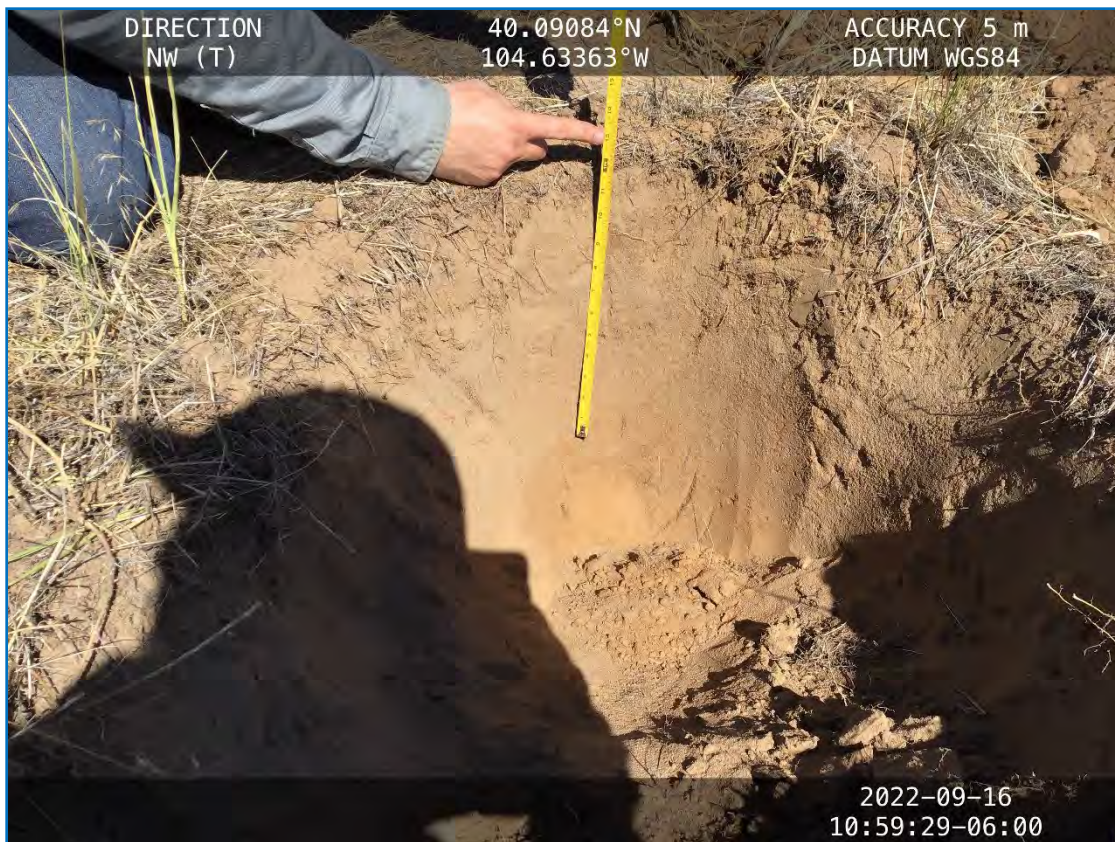
Photograph 5. Topsoil depth pit (S05); showing transition to orange, more compact soil at approximately 13 inches. Soil sandy throughout pit.
