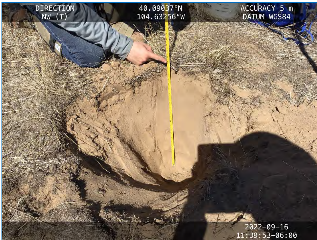
Photograph 7. Topsoil depth pit (S07); depth greater than 2 feet. Soil sandy throughout pit, with no change in color or texture.
