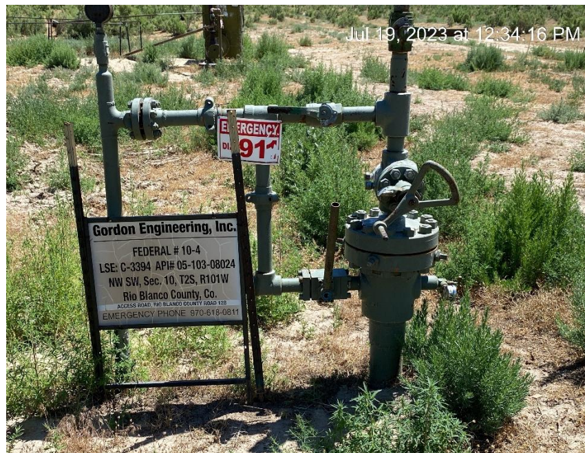
Wellhead with no Bradenhead access
