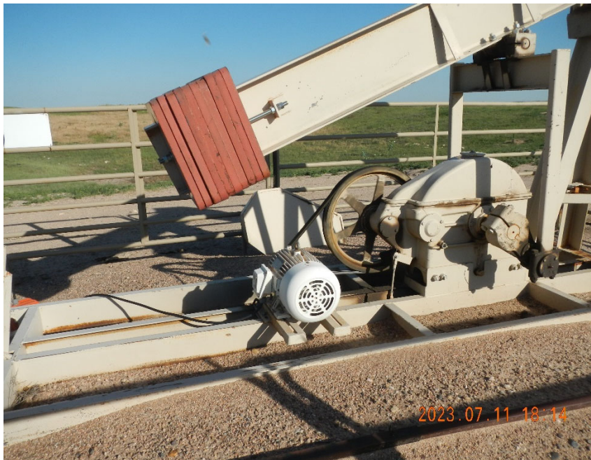
3. View of Pump Jack with Electric Motor.
