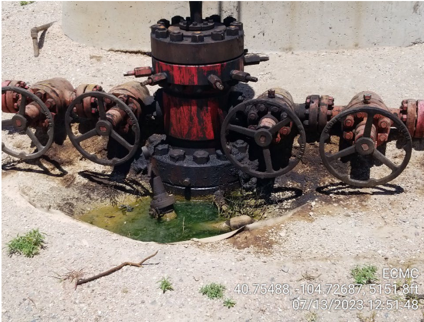
Photo 7 – Wellhead – Stained Soil
