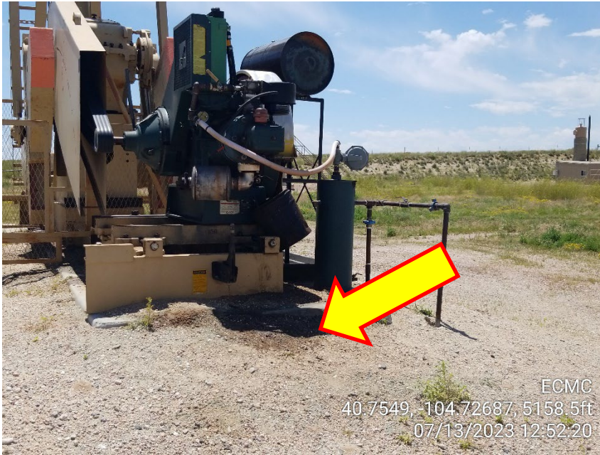
Photo 9 – Gas Engine – Stained Soil
