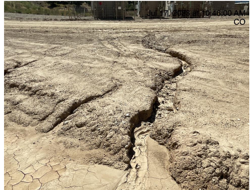
Photo # 3277 Rill erosion (N/NE area of location)
