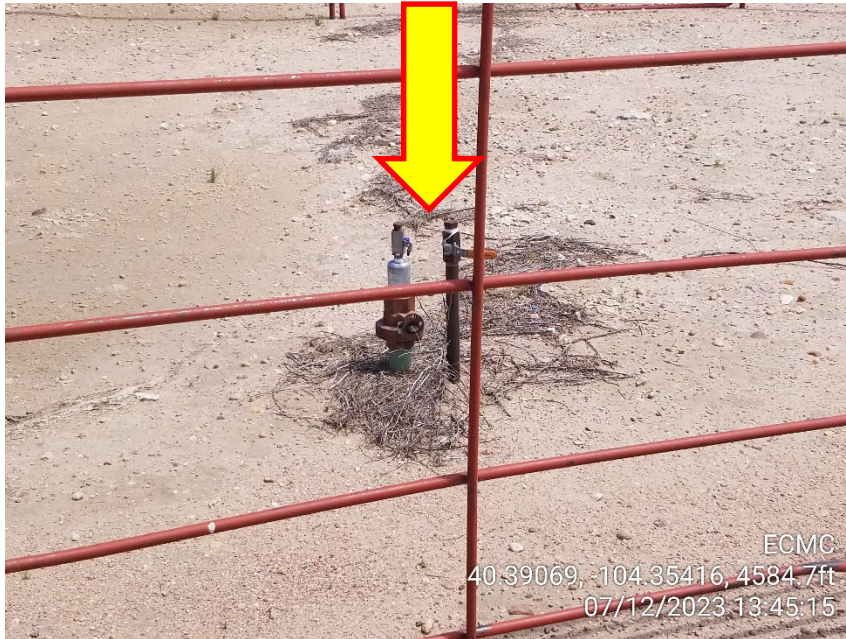
Photo 3 – Unmarked Risers at Wellheads
