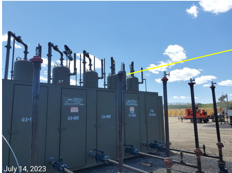
Photo 4: Uncapped/exposed line observed at separator equipment.
