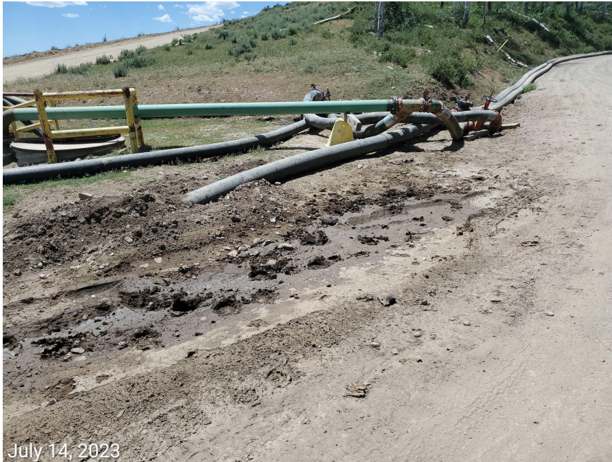
Photo 6: Spill observed at frac lines south of the Location.
