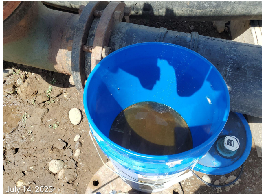
Photo 7: Spill observed at frac lines south of the Location. Fluids observed leaking into the blue bucket containing dark fluids.
